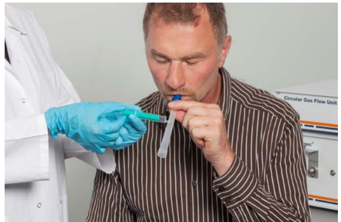
Figure 1: Manual sampling option: Exhaled breath is sampled into a reservoir (syringe) and afterwards manually injected into the device (figure 2).
