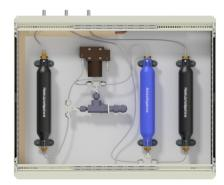
Technical drawing of the CGFU. Two molecular sieves and an activated carbon filter clean the circulating air to a high grade.
