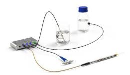
This single-device solution for multi-analyte measurements has integrated atmospheric pressure and humidity sensors for precise and easy oxygen sensor calibration, but also for automatic pressure compensation of the oxygen measurements. Furthermore, the *FireSting pro* offers 4 analog outputs and a broadcast-mode.
