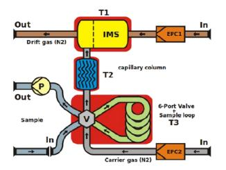
Figure 2: General set-up of the GC-IMS instrument.
