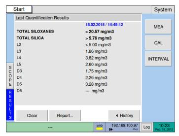
**Figure 8:** Results window of the GC-IMS SILOX. Concentration of siloxane species L2-L5 and D3-D5 are displayed just as the calculated concentration for total siloxanes and silica.
