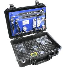
The Gaseous Fuels Sorbent Tube Sampling System was specifically designed for natural gas, biogas and other gaseous fuels. It can be used with a variety of sorbent tubes/traps, including Siloxanes, Hg, HCl, HF, and NH<sub>3</sub>. Simply insert two sorbent tubes/traps, record the barometric pressure and temperature, open the sample valve, set the flow rate, start the timer and wait for the desired sample time to be achieved.
