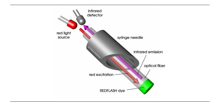
The measuring principle is based on a sinusoidally modulated red excitation light. This results in a phase-shifted sinusoidally modulated emission in the NIR. The **PyroScience** read-out device measures this phase shift (termed "**dphi**" in the software). The phase shift is then converted into oxygen units based on the Stern-Vollmer-Theory.
