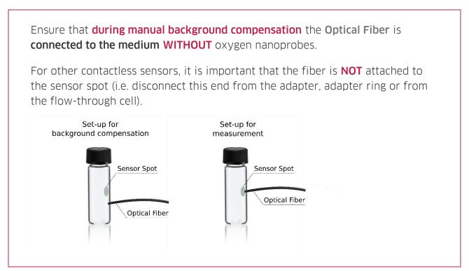
Please ensure that **during the subsequent calibration process** the **Optical Fiber** is again **attached to the medium WITH** oxygen nanoprobes or to the position with sensor spots.
