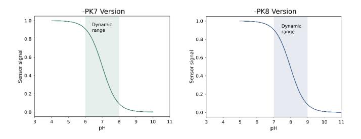
Calibration of both versions is performed at low pH values (completely protonated indicator dye) and at high pH values (completely de-protonated indicator dye). For this reason, it is possible to use the same pH buffer capsules (**PHCAL2** and **PHCAL11**) for both pH sensor versions.
