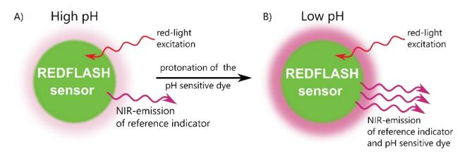
**Principle:** red light excited REDFLASH sensor shows luminescence in the near infrared (NIR). The REDFLASH sensor consists of a pH insensitive reference indicator and a pH sensitive dye.**A**) low NIR emission from just the reference indicator and **B**) high NIR emission from the protonated dye and the reference indicator.
