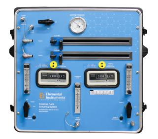
The Ei310 Series Gaseous Fuels Sampling System was specifically designed for natural gas, biogas, and other gaseous fuels. It can be used with a variety of sampling methods, including sorbent tubes/traps, sampling bags, cylinders, canisters, and EPA Method 29 and MIC sampling trains.
