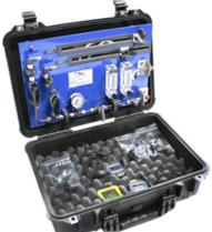
The Gaseous Fuels Sorbent Tube Sampling System was specifically designed for natural gas, biogas and other gaseous fuels. It can be used with a variety of sorbent tubes/traps, including Siloxanes, Hg, HCl, HF, and NH<sub>3</sub>. Simply insert up to two sorbent tubes/traps, record the barometric pressure and temperature, open the sample valve, set the flow rate, start the timer and wait for the desired sample time to be achieved.
